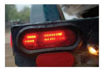
**More blinkety-blink LEDs.** The left tail light on the same boat trailer hasn't fared much better than the right. Although it has two rows of LEDs working, neither is a full row. The owner is faced with having to already replace tail lights again in less than two years.
