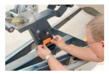
**Won't pass as Rudolph.** But the amber reflector on the trailer's bow stop area serves to illuminate an otherwise dark area of the trailer when hit by headlights, whether passing through an intersection or sitting idle in a boat ramp parking lot.
