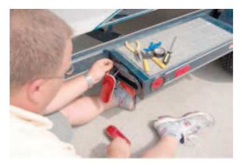
**Oval grommet tail lights a snap to replace.** Any adept handyman or woman can install a replacement Optronics trailer light without problem. Each replacement kit comes with the sealed light insert, rubber grommet and pigtail.
