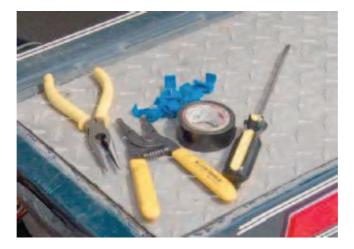
**Only basic tools needed.** A pair of needlenose pliers, wire cutter/stripper, wire connectors or nuts, screwdriver and electrical tape are all you need to install most Optronics replacement light kits.
