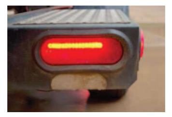
**All LED trailer lights are not created equal.** A partial single row of LEDs is all that remains working on this boat trailer's "waterproof" right
