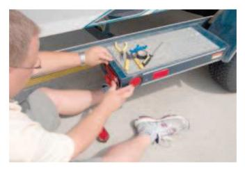
**That's all there is to it.** Connect the pigtail to the trailer's wire using wire connectors or wire nuts. Plug the pigtail into the back of the LED cartridge. Fit the cartridge into the rubber grommet. Done!
