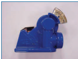
Powder Coated - Minimal corrosion where scored
