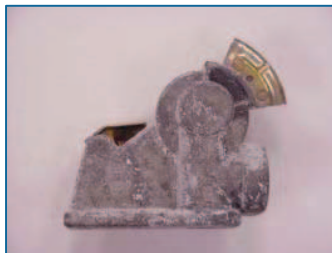
Standard - Heavy corrosion on entire body
