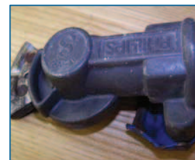
Anodized - Virtually no corrosion on the body
