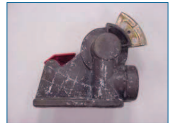
Anodized - minimal corrosion where scored
