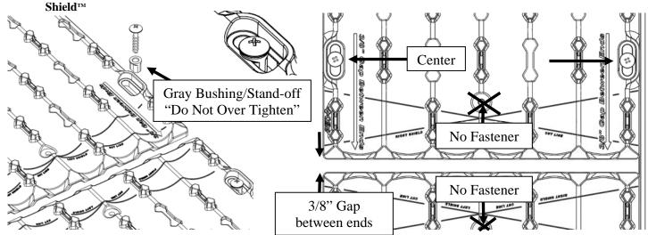
**NOTE:** The screws supplied with this kit are not meant to be used in steel or aluminum, but can be if an 11/64" drill bit is used first to drill a pilot hole. Caution should be used in areas where marker lights and wires have been installed under the trailer deck when installing all fastener.
