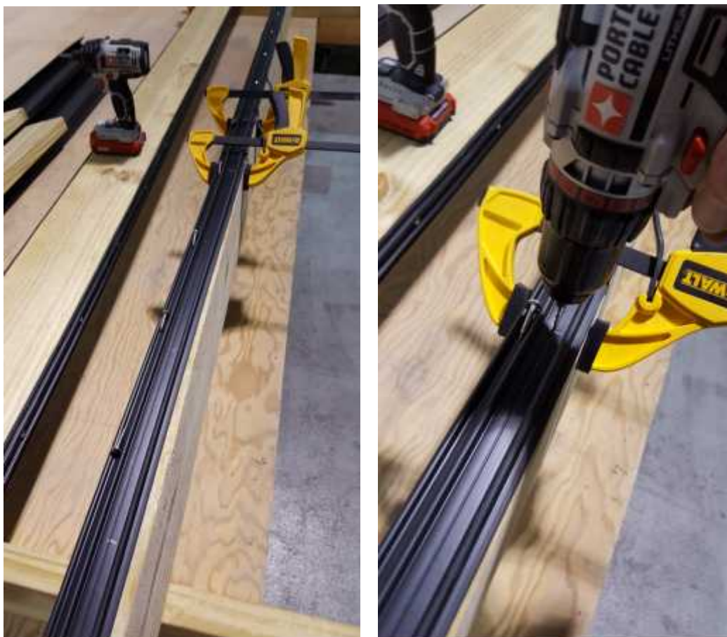
FIG 4 Screw placements are marked and screws are installed. Right, you can see a Drill being used to Pre-Drill a location for a screw. Use a smaller drill bit to allow the screws to grip properly when installed.
