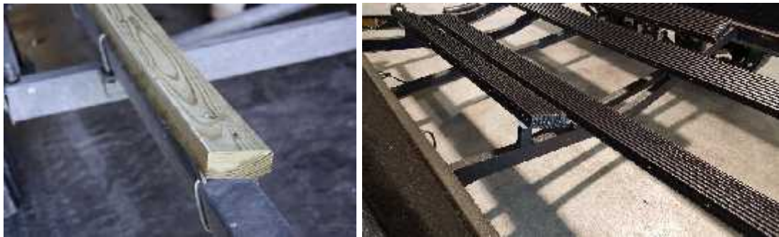
FIG 1.3 Decide if you will replace bunk covers on or off the trailer
